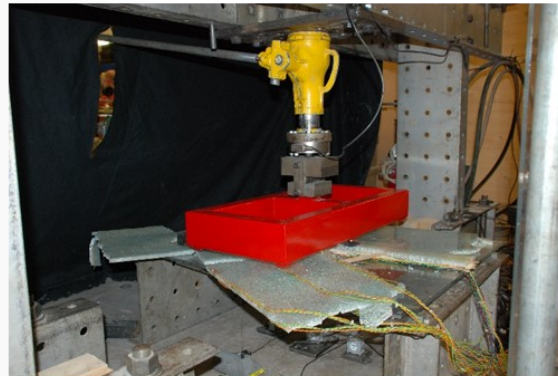
Fig. 2. Four-point bending test on composite panel
