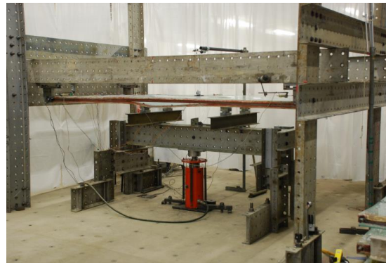
1 | Bending test on 3.5 x 1.5 m 2 composite glass panel
