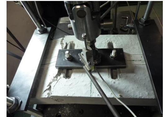
2 | Experimental testing of steel connection in UHPC material
