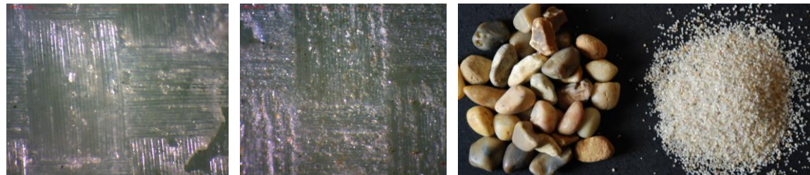
1 | Surface finish prior and post sand abrasion (left), abrasion medium (right)
