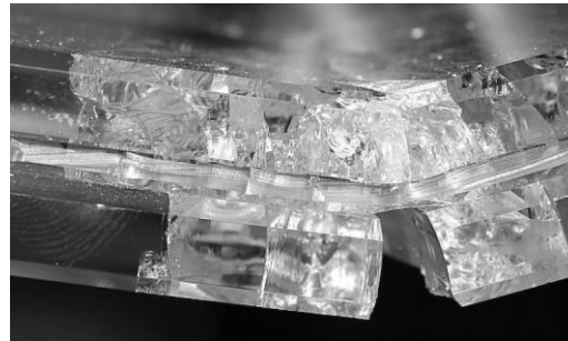
1 | Plastic hinge developed in laminated glass beam following the fracture of both glass layers (Delincé et al., 2008)
