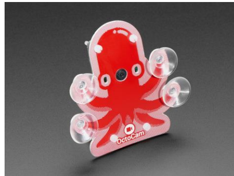
1 | Octocam. A raspberry PI that captures images
