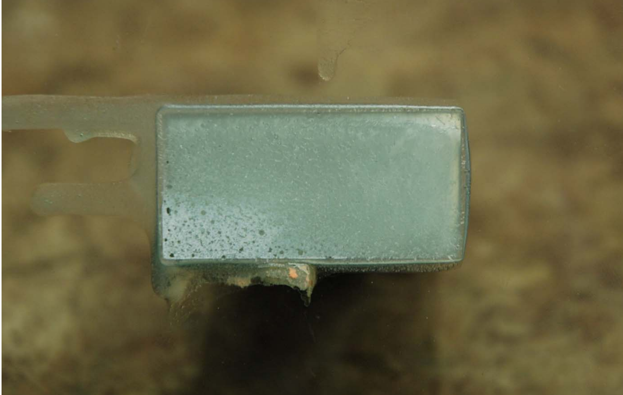
Figure C3 - Typical Failure of T-Peel Bohle Sample
