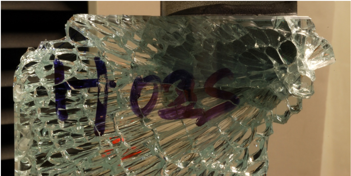
Figure C4 - Failure of Glass in a Holdtite Sample
