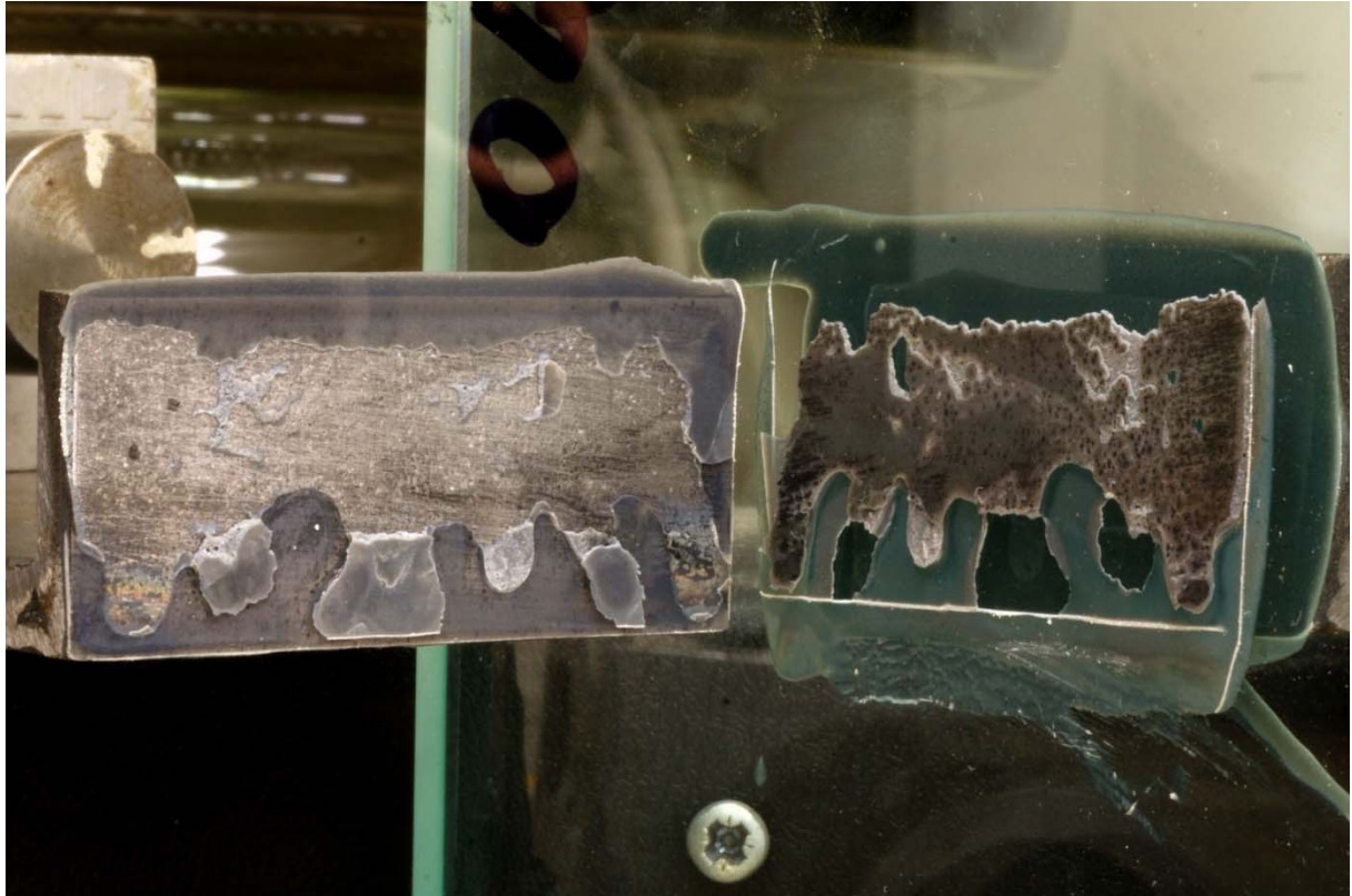
Figure C5 - Failure of 3M T-Peel Sample
