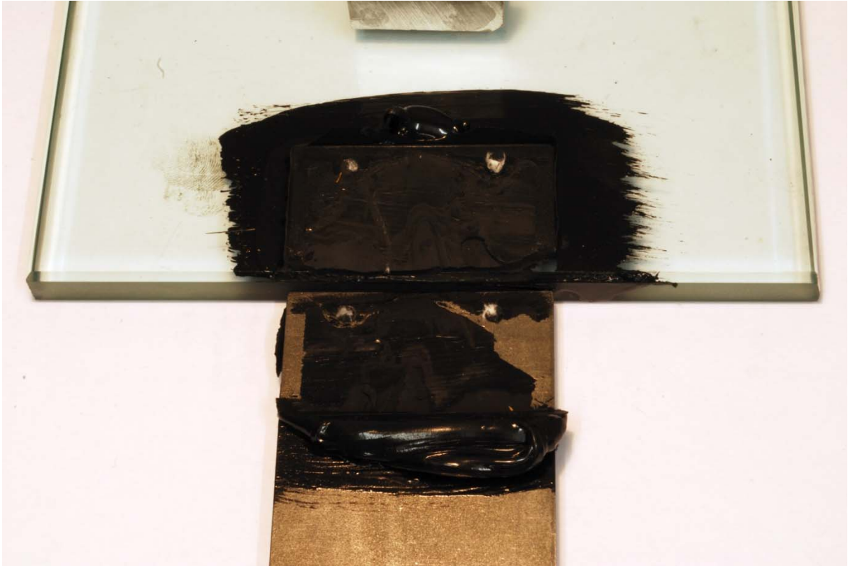
Figure C2 - Adhesive Failure in SikaForce
