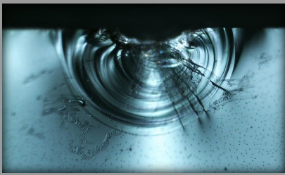
Micrograph of critical flaw in glass.
