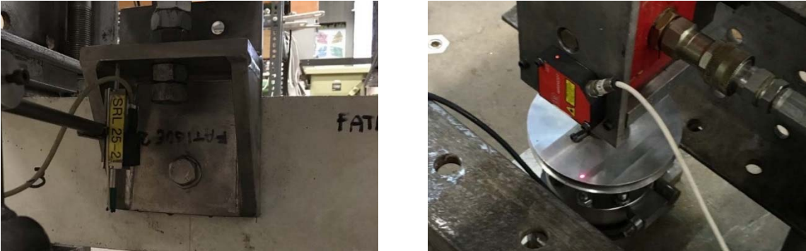
Figure 6. Linear potentiometer displacement transducer (left) and Detail of the laser displacement transducer (right)
